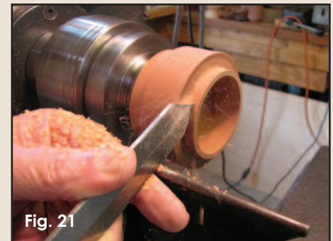
Fig. 21 Carefully adjust the tenon for a jam fit.
