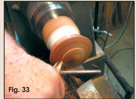
Fig. 33 Shape the bottom so that the curve mirrors the top.
