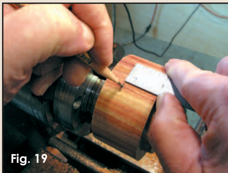
Fig. 19 Measure and mark the body height on the blank.
